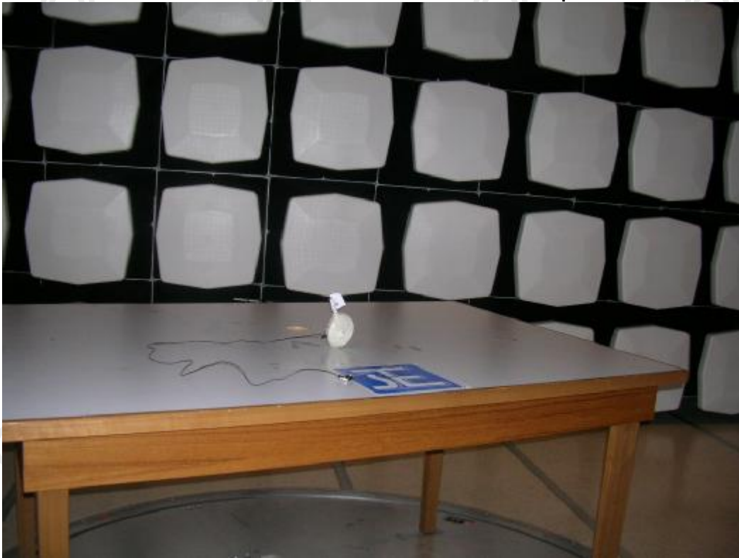
Measurement of Radiated Emission Test Set Up
