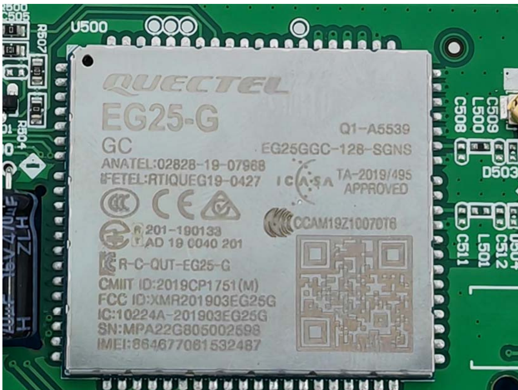
WWAN Module, FCC ID: XMR201903EG25G IC: 10224A-201903EG25G
