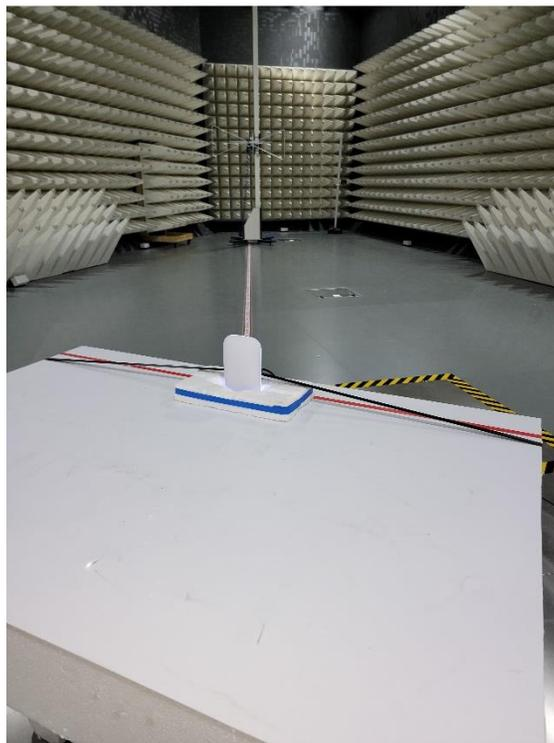
**Photograph 1: Test Set Up Radiated Emissions 30 – 1000 MHz**
