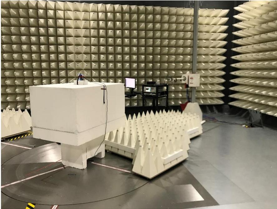
**Photograph 3: Test Set Up Radiated Emissions 17 - 40 GHz**
