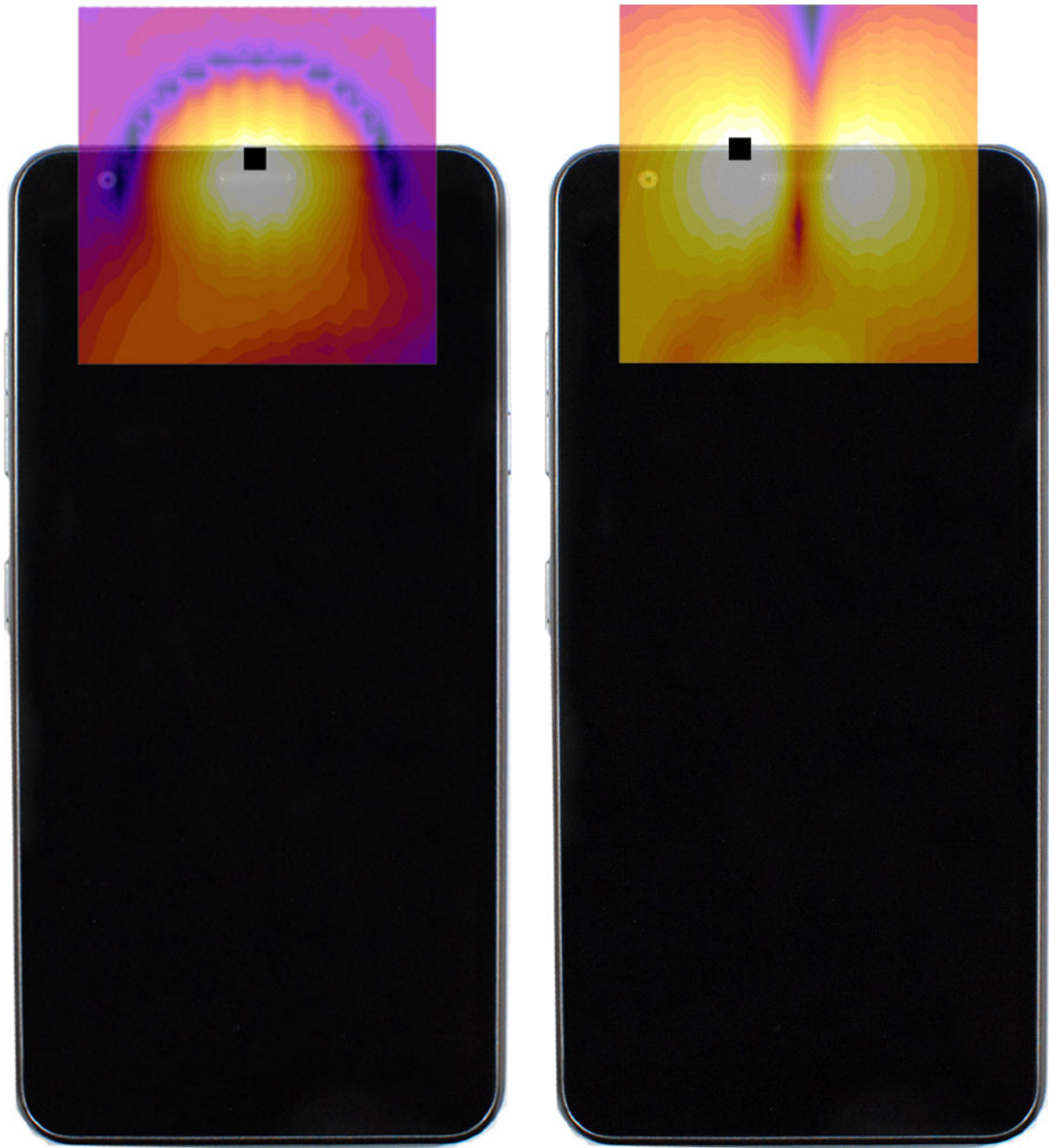
Figure 16-3 T-Coil Scan Overlay Magnetic Field Distributions
