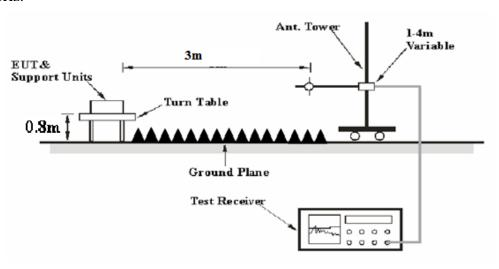
The radiated emission below 1GHz tests were performed in the 10 meters chamber test site, above 1GHz tests were performed in the 3 meters chamber test site A, using the setup accordance with the ANSI C63.4-2014. The specification used was with the FCC Part 15 B Class B limits.
