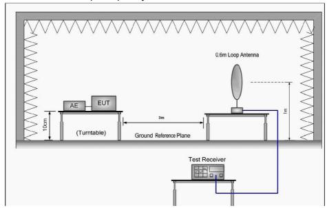
(B) Radiated Emission Test-Up Frequency 30MHz~1GHz
