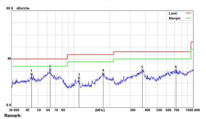
Measurement Level= ReadingLevel+ Factor, Margin= Measurement Level - Limit
