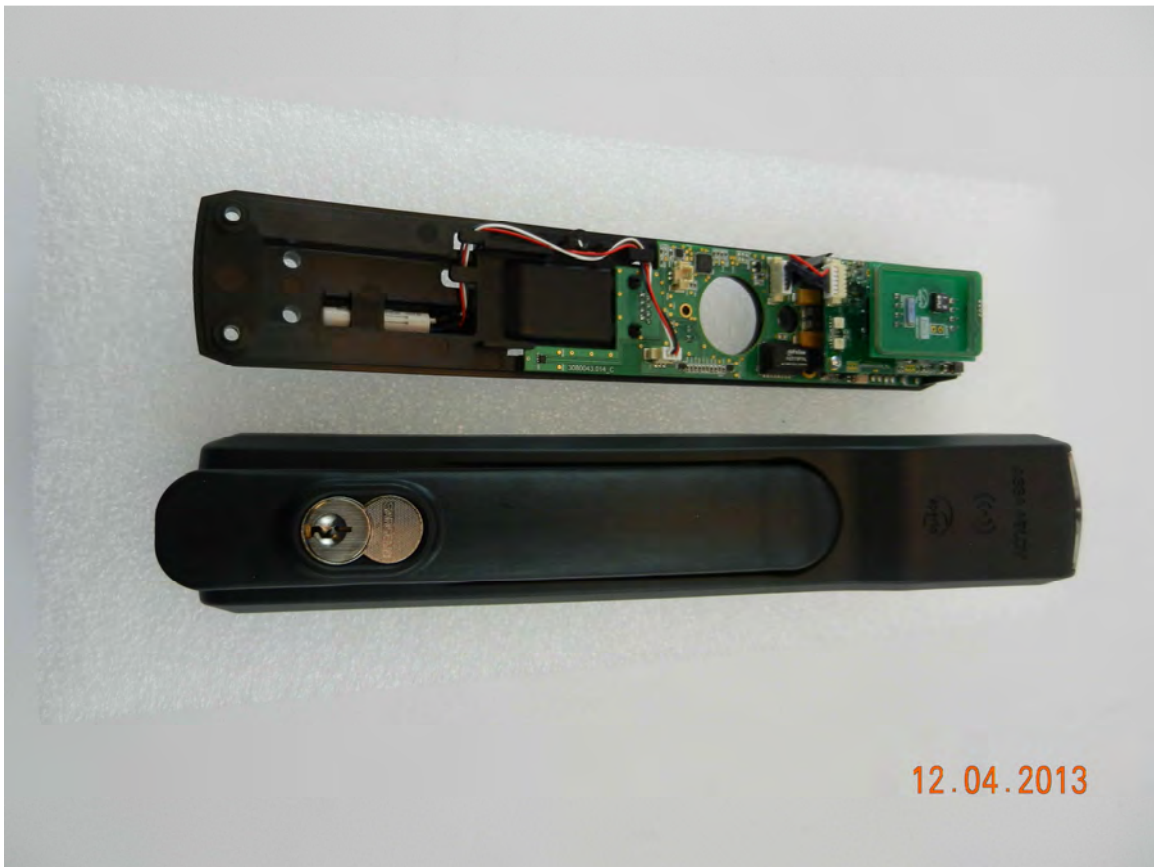
Assembled back plate next to front cover
