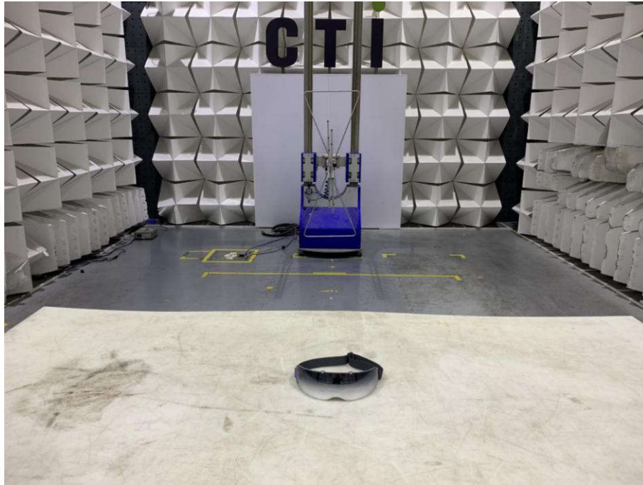
Radiated spurious emission Test Setup-1(Below 1GHz)
