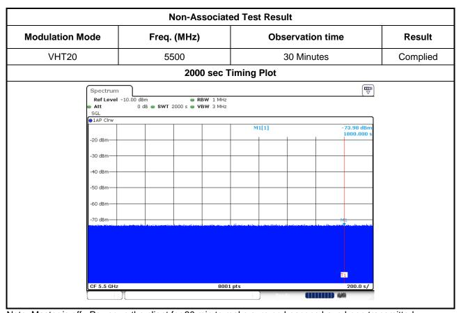
Note: Master is off. Power up the client for 30 min to make sure no beacons have been transmitted
