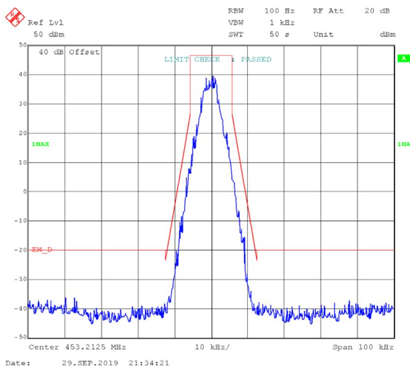
**4FSK,12.5kHz, Low Power - Frequency 453.2125 MHz:****99% Occupied & 26 dB Bandwidth**
