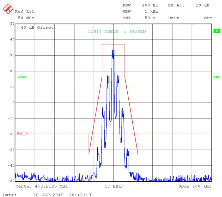
**4FSK,12.5kHz, High Power - Frequency 453.2125 MHz:****99% Occupied & 26 dB Bandwidth**
