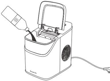
3. Use the water to rinse the inside parts and drain out the water by unplugging the drain cap on the front bottom side.
