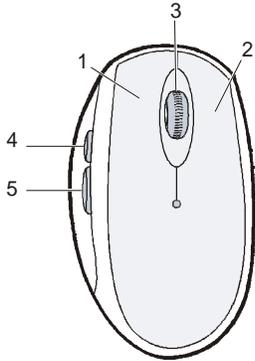
There are two additional 4 and 5 on left side on mouse. The two buttons are using in page-up and page-down on acquiescence operating system. You can set-up this two button as you like when installing CD driver.
