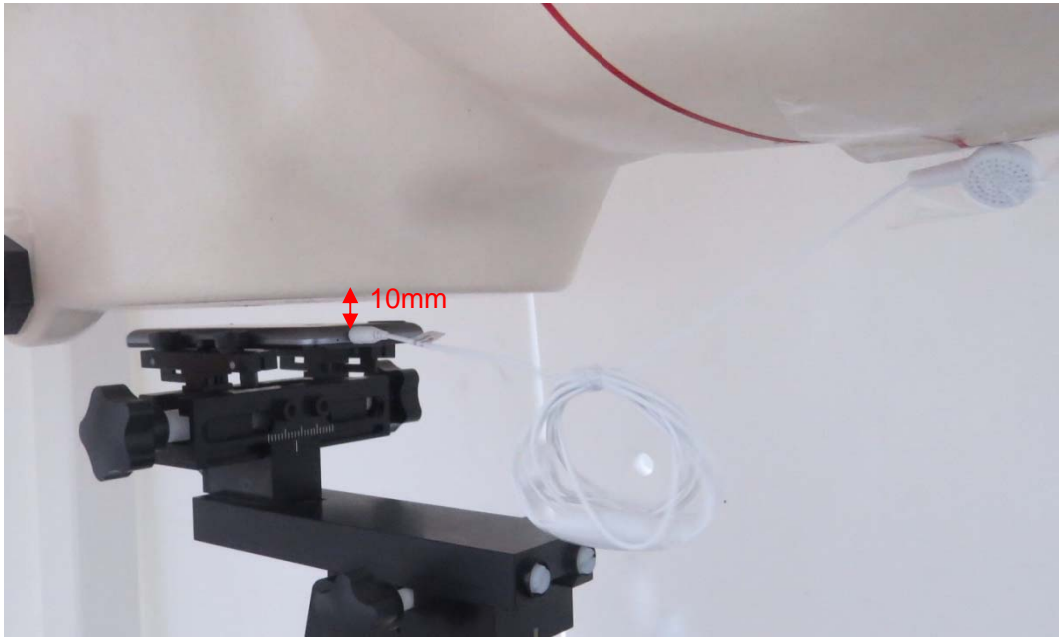
Picture 13: Back Side with Earphone 2, the distance from handset to the bottom of the Phantom is 10mm
