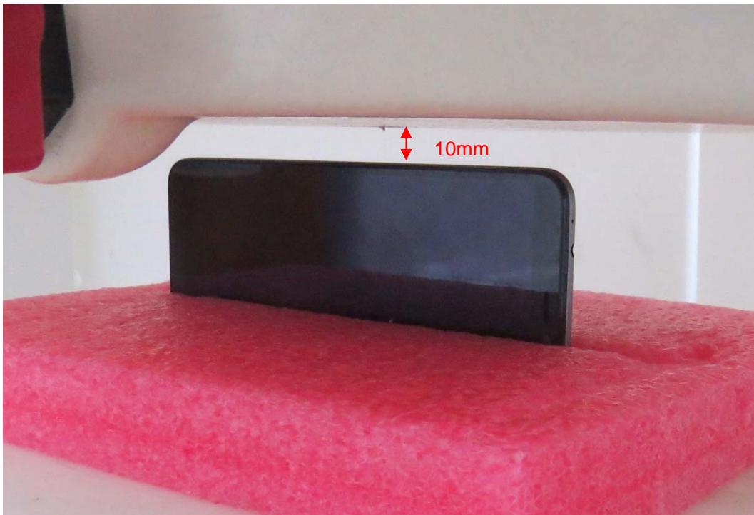
Picture 8: Left Side, the distance from handset to the bottom of the Phantom is 10mm
