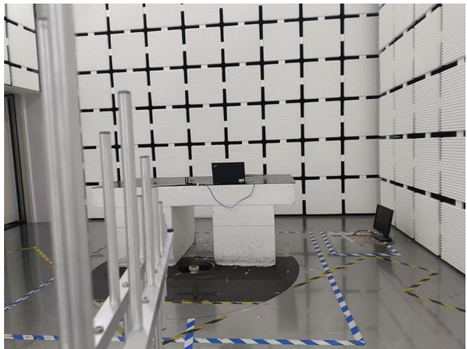
Radiation Emission Test Setup (30MHz to 1GHz)
