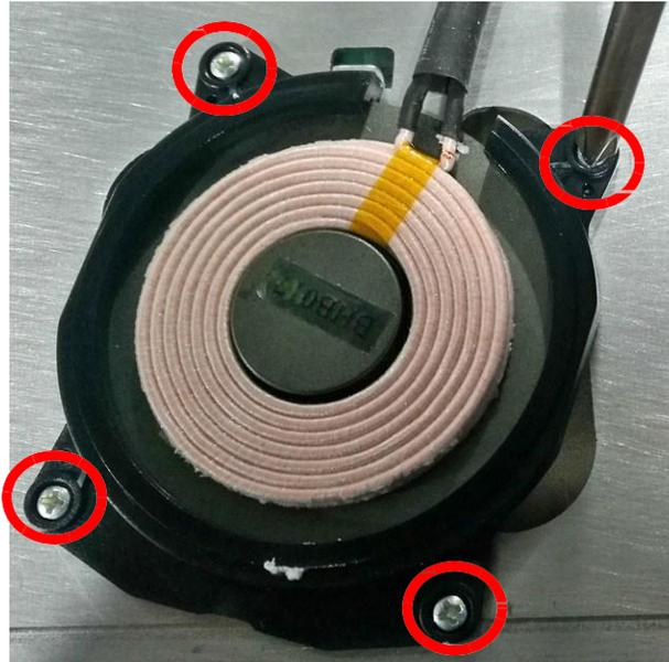
6. Replace the coil module with new one and re-install it on the frame.
