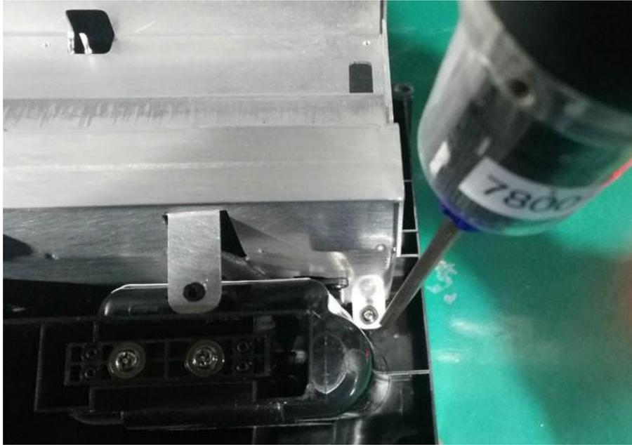
5. Remove the four screws between the coil module and the frame.
