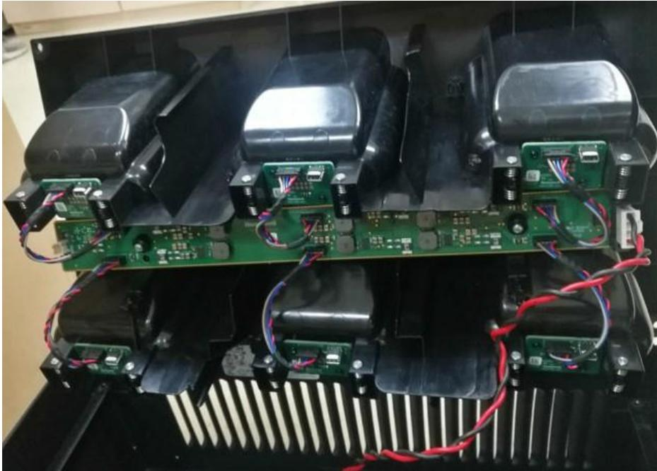
**Pull the bay out and rotate it to the right to access cables.**
