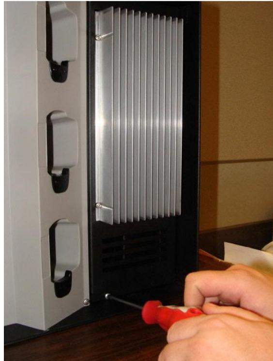
19. The installation should be complete. Re-install the AC cord and test for functionality.
