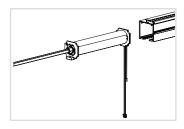
**Step 5.** Ensure power cord and antenna extend freely from the headrail. Anchor the Motor to the headrail.
