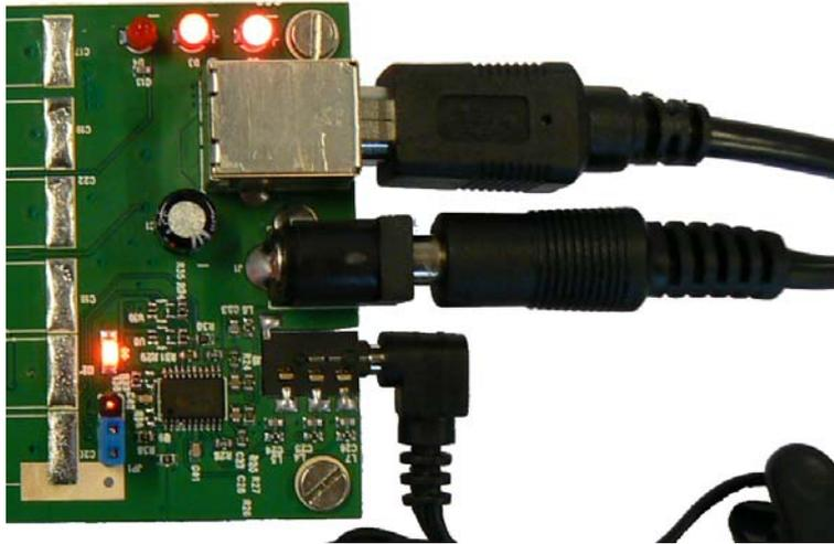
**Figure 5: Top to bottom: USB cable, power plug and audio jack**
