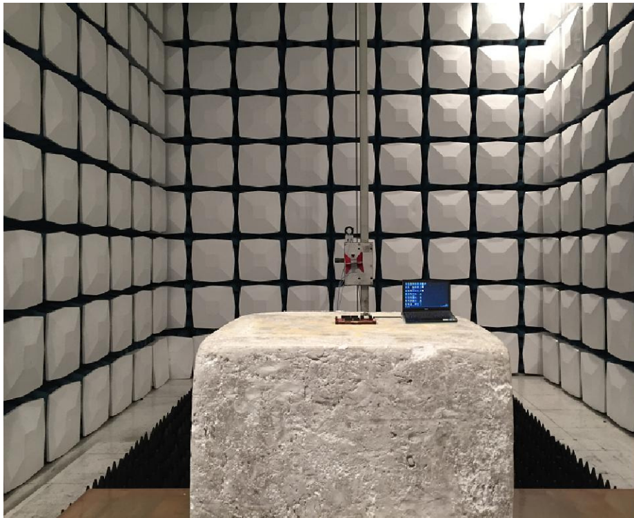
Description: Radiated Emission Test Setup for 1~18GHz
