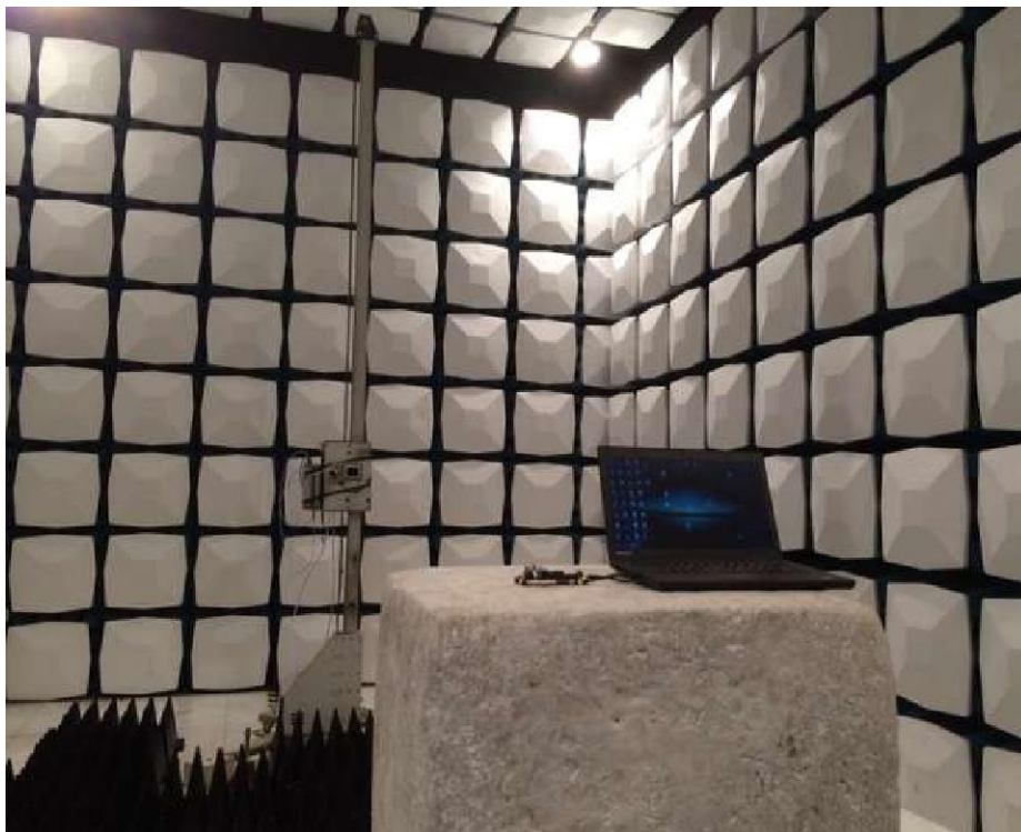
Description: Radiated Emission Test Setup for 18~40GHz
