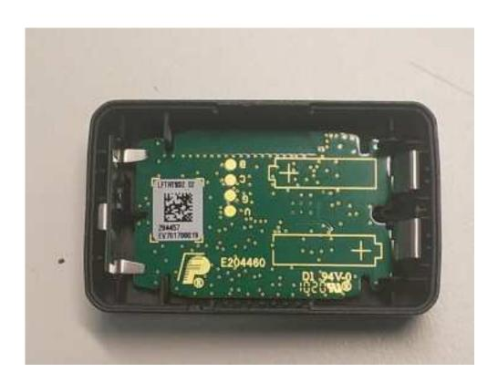
Snap the B cover in place (please note that the B cover can be placed only in one direction). The device starts making distance measurements about any objects on the top side of the device. Measurements are made once a minute (default, can be changed by configuration).
