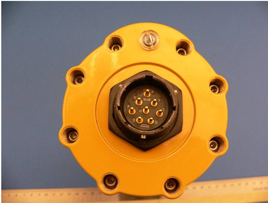
EUT – IO Connector 1
