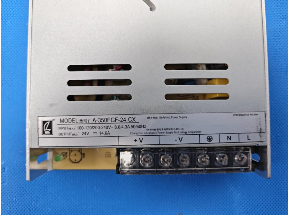
Power supply model: A-350FGF-24-CX
