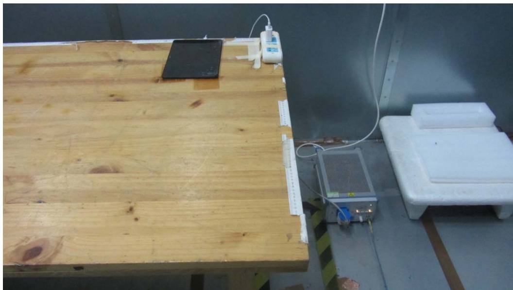
Picture 2 Conducted Emission Test Setup
