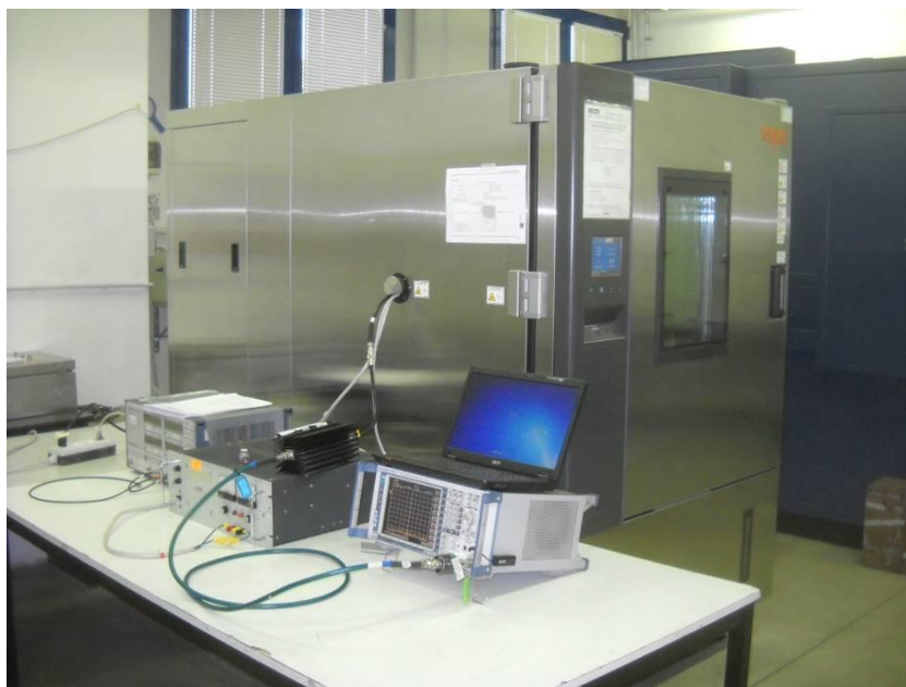
Set-up photo for frequency error tests
