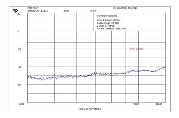
$f < 1 \ GHz: RBW/VBW: 100 \ kHz \\ Carrier suppressed with a rejection filter. \\ f \geq 1 GHz: RBW / VBW 1 \ MHz$
