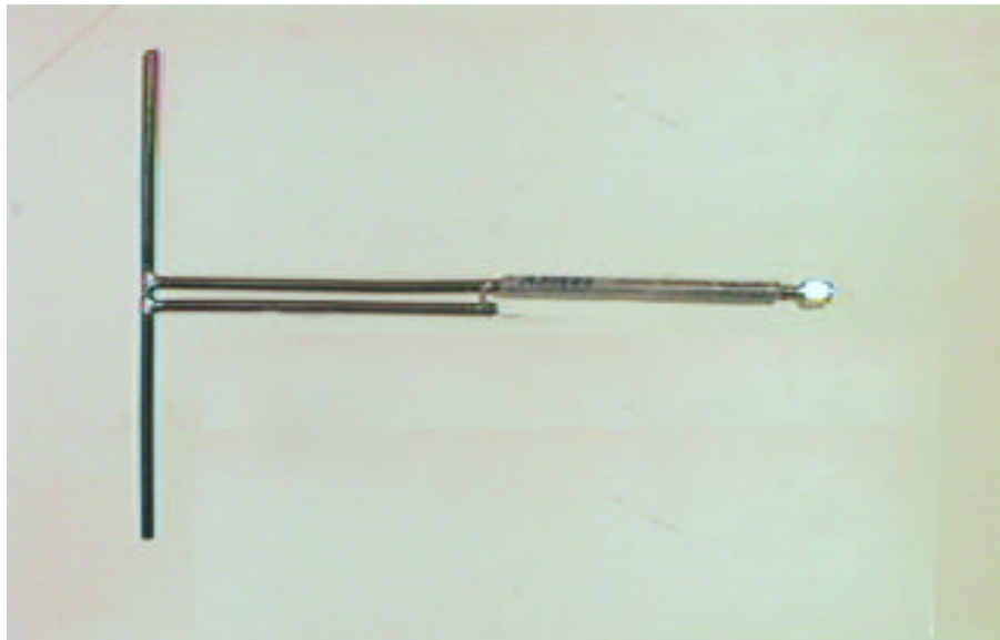
Reference Dipole Antenna Used for ERP Measurement
