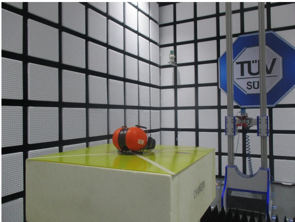
Radiated Emission Test above 1 GHz
