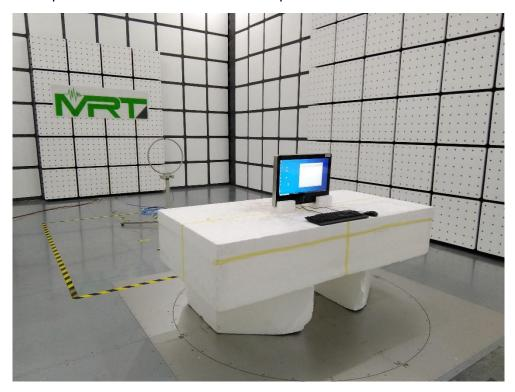
Description: Radiated Emission Test Setup for 30MHz~1GHz
