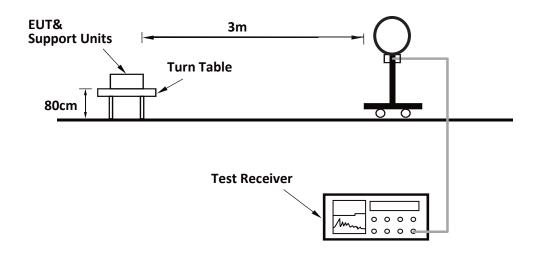
For Radiated emission 30MHz to 1GHz:
