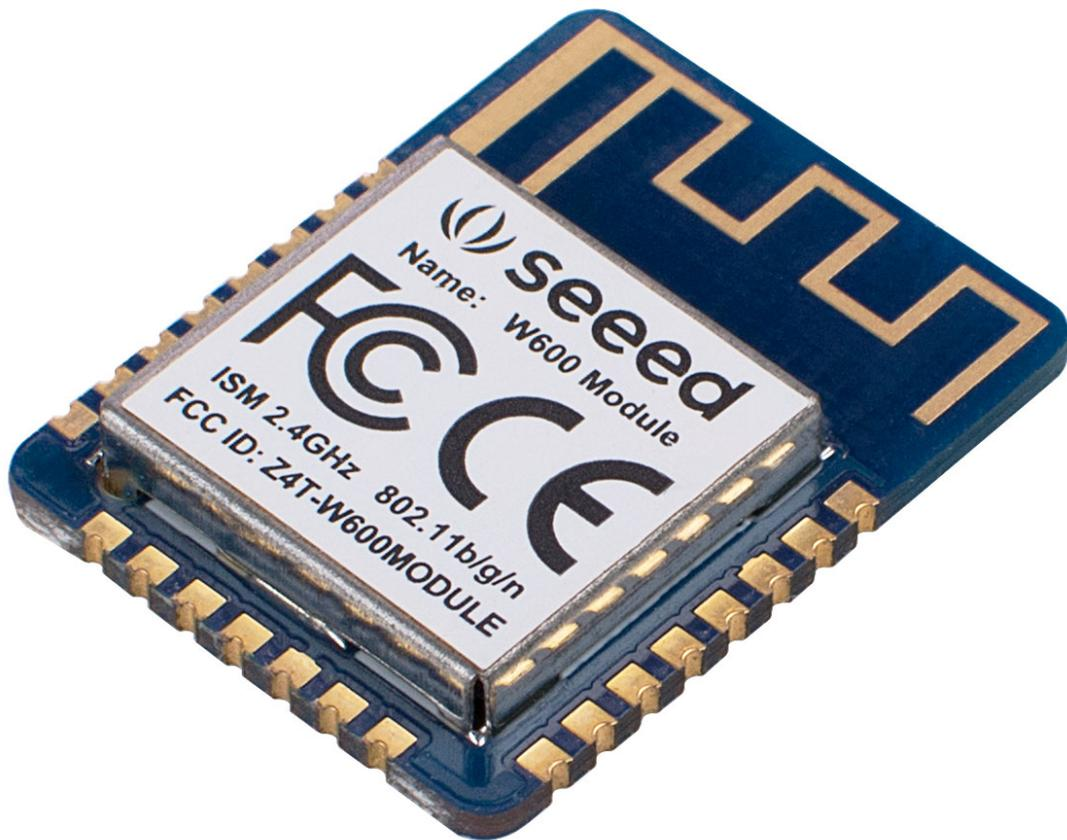
The W600 Module is a cost-effective 2.4GHz WiFi module support 802.11b/g/n. Seeed W600 Module is based on the W600 chip which features ARM Cortex-M3 with 1MB on-chip flash and freeRTOS kernel.
