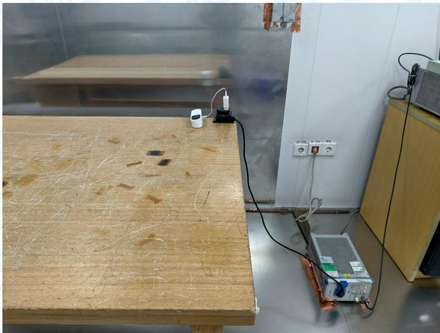
Photo of Setup for Conducted Emission
