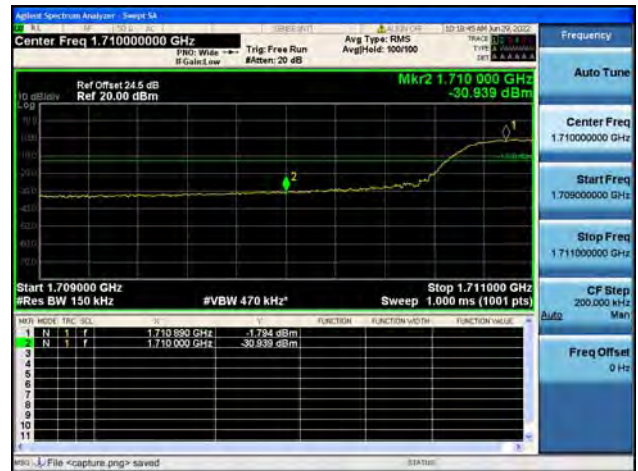
B66 / 15MHz / High CH / QPSK / FULL RB
