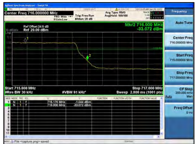
B12 / 3MHz / High CH / QPSK / FULL RB
