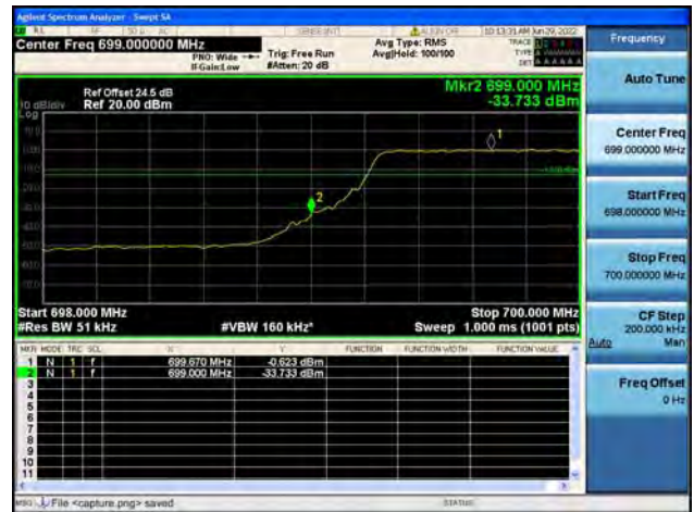
B12 / 5MHz / High CH / QPSK / FULL RB
