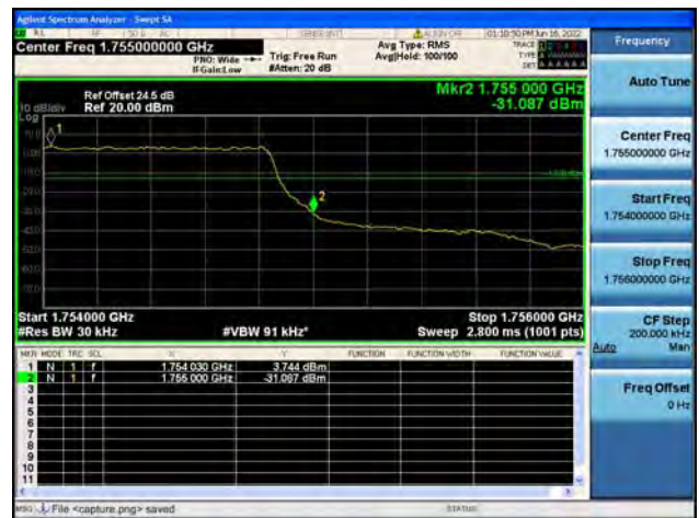
B4 / 1.4MHz / High CH / QPSK / FULL RB
