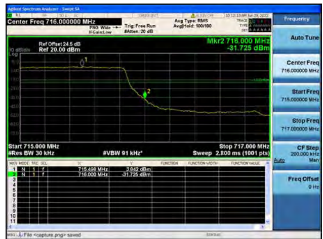
B12 / 1.4MHz / High CH / QPSK / FULL RB
