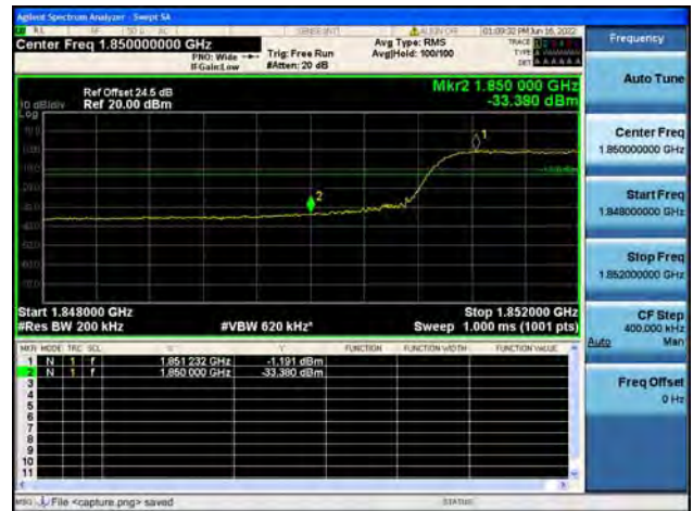
B2 / 20MHz / High CH / QPSK / FULL RB
