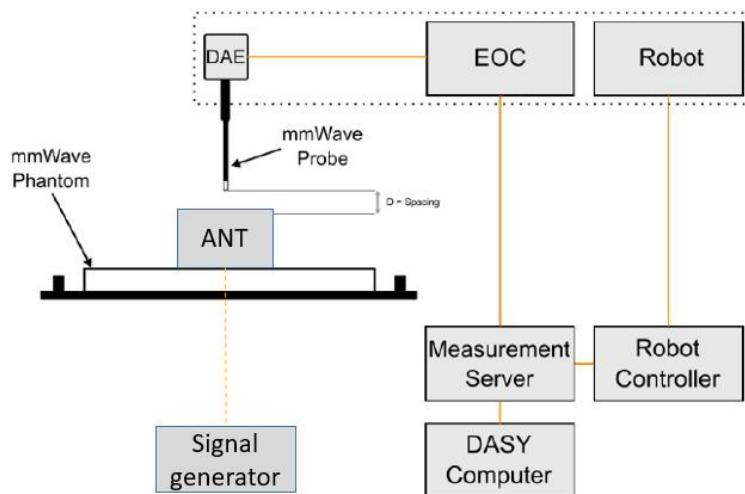
Note: Measurement accuracy can be reduced if connected to a ground pin at the backside of the robot arm. Create a measurement file with a test distance of 10mm for 10 GHz and 5.55mm (Horn build inside and 4.45mm to the outer surface) for 30 GHz and above. The sources at 30 GHz and above comprise horn antennas and very stable signal generators. The 10 GHz horn antenna has a SMA connector and can be connected to any signal generator.
