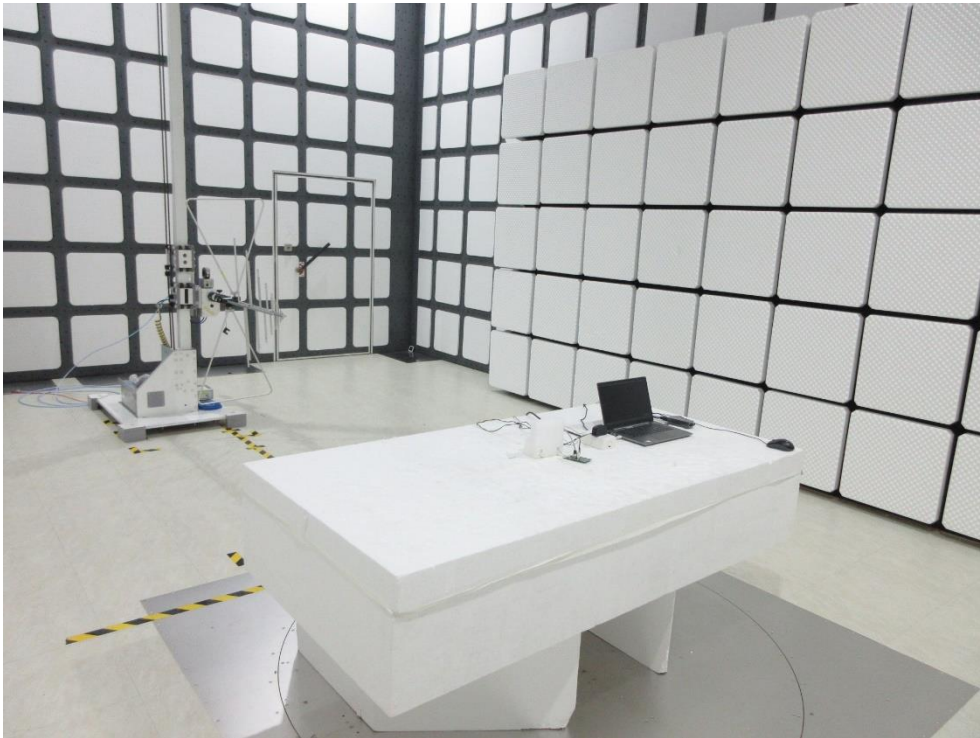
Description: Radiated Emission Test Setup for 1GHz~18GHz
