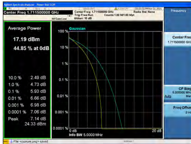
Band66 / 3MHz / Mid CH / QPSK
