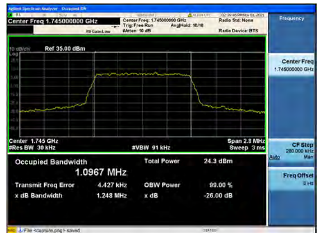
Band66 / 1.4MHz / High CH / 16QAM
