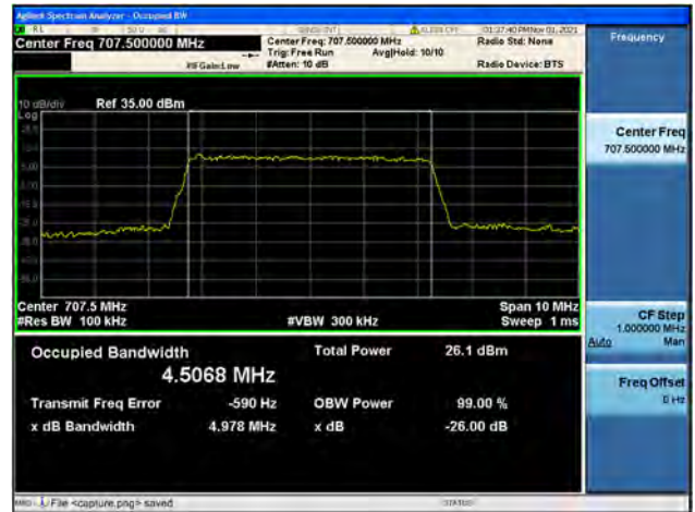
Band12 / 5MHz / High CH / 16QAM
