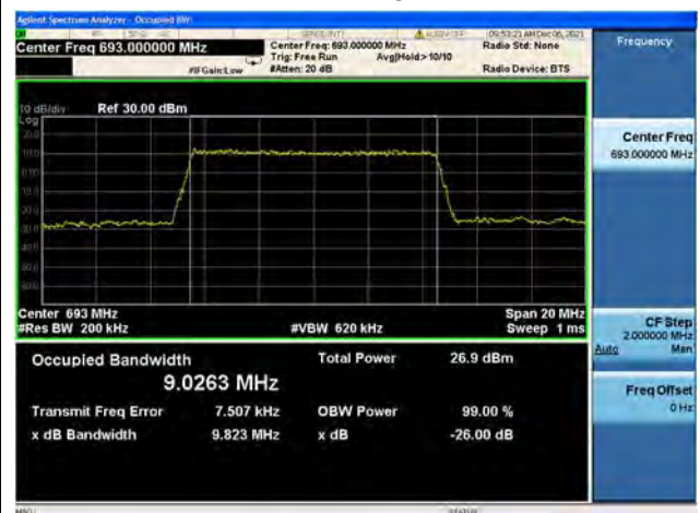
Band71 / 10MHz / High CH / 16QAM
