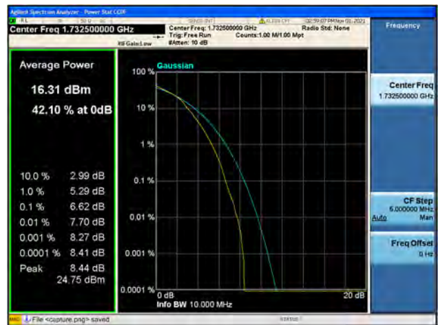
Band4 / 10MHz / High CH / 16QAM
