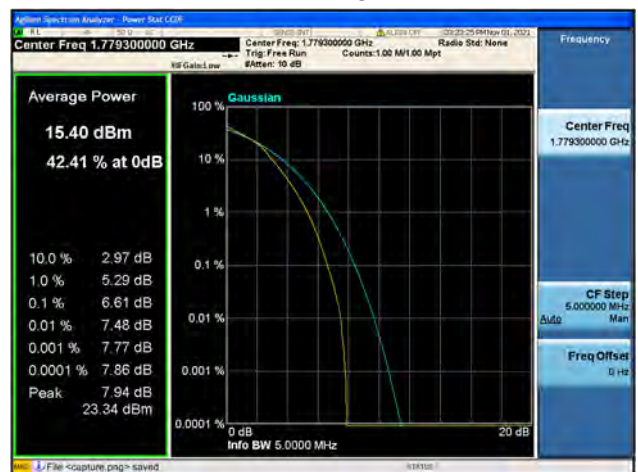
Band66 / 1.4MHz / High CH / 16QAM
