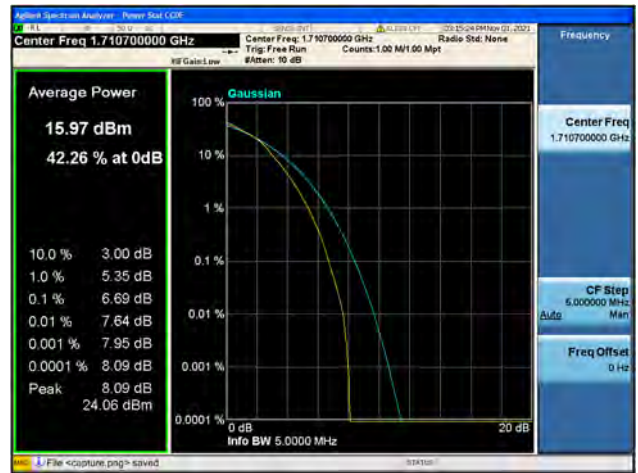
Band66 / 1.4MHz / Mid CH / 16QAM
