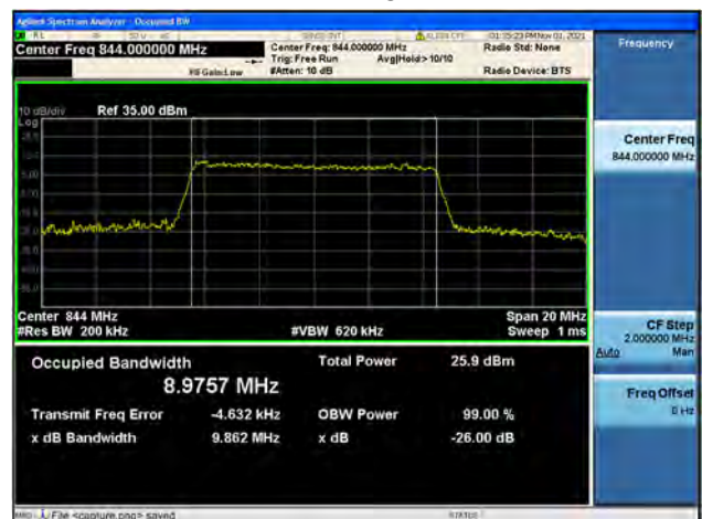
Band5 / 10MHz / High CH / 16QAM
