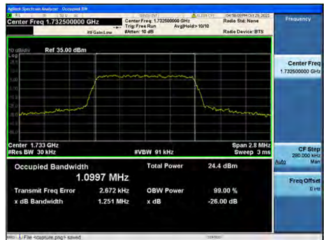
Band4 / 1.4MHz / High CH / 16QAM
