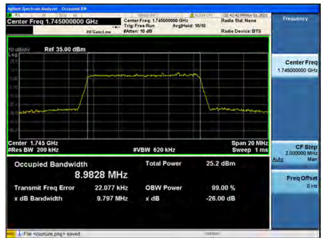
Band66 / 10MHz / High CH / 16QAM
