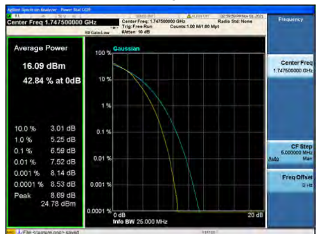
Band4 / 15MHz / High CH / 16QAM
