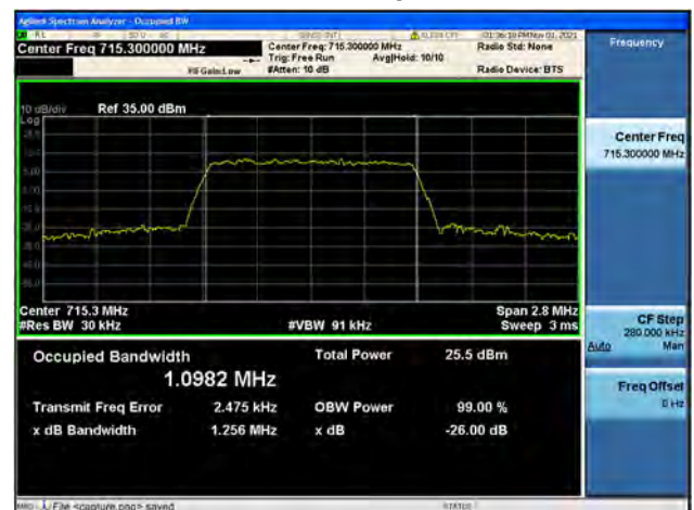
Band12 / 1.4MHz / High CH / 16QAM
