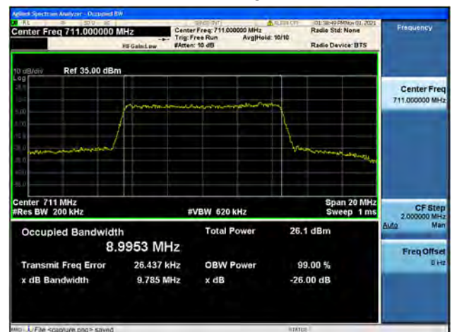
Band12 / 10MHz / High CH / 16QAM
