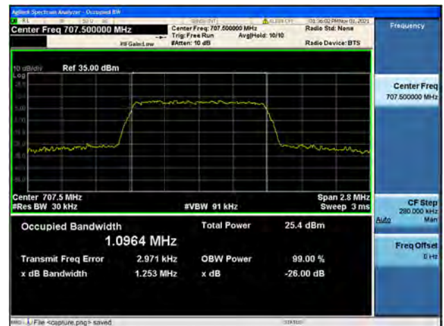
Band12 / 1.4MHz / High CH / 16QAM
