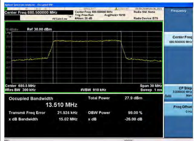
Band71 / 15MHz / High CH / 16QAM
