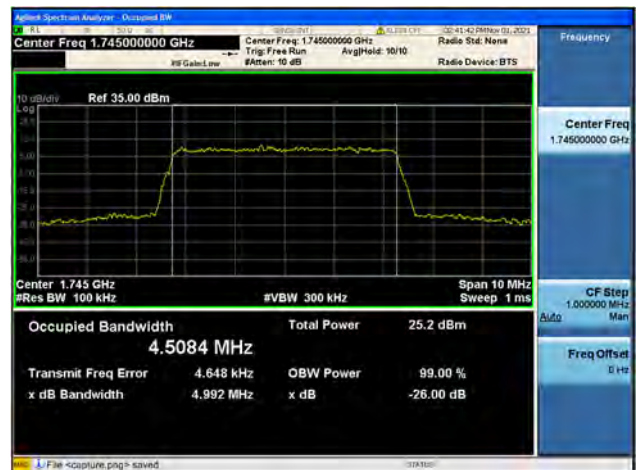
Band66 / 5MHz / High CH / 16QAM
