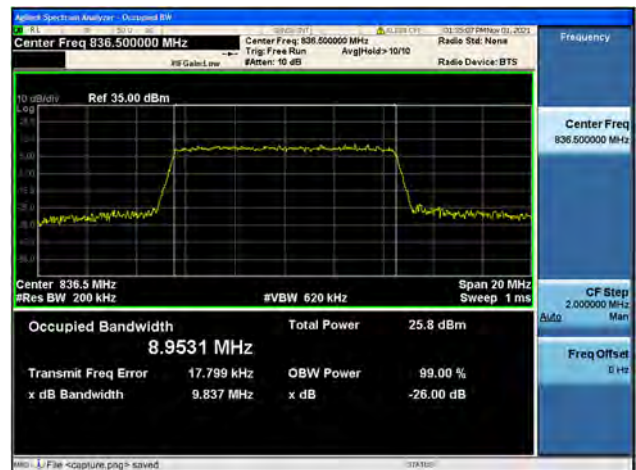
Band5 / 10MHz / High CH / 16QAM
