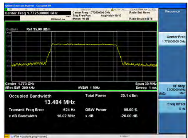
Band66 / 15MHz / High CH / 16QAM
