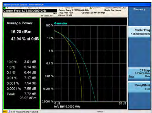
Band4 / 5MHz / High CH / 16QAM
