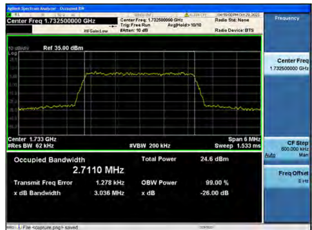
Band4 / 3MHz / High CH / 16QAM
