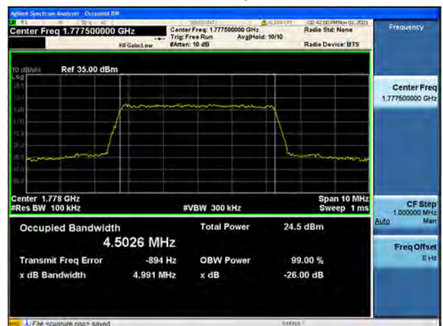
Band66 / 5MHz / High CH / 16QAM
