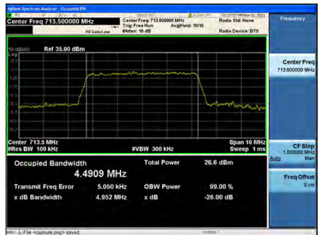
Band12 / 5MHz / High CH / 16QAM
