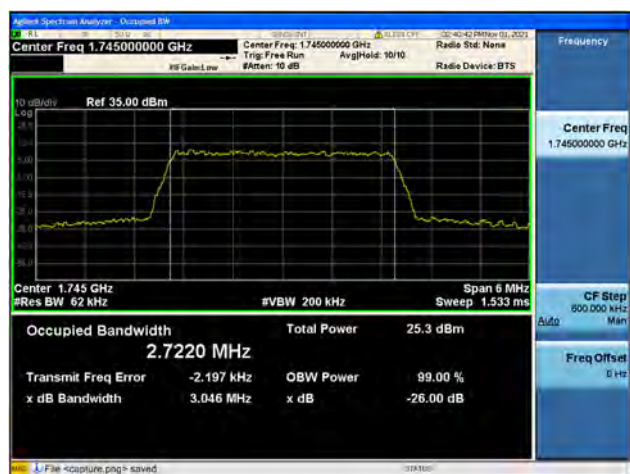
Band66 / 3MHz / High CH / 16QAM
