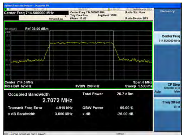
Band12 / 3MHz / High CH / 16QAM
