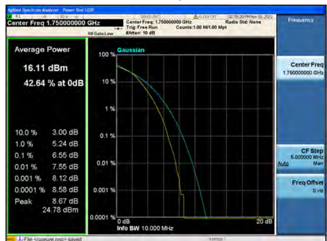
Band4 / 10MHz / High CH / 16QAM
