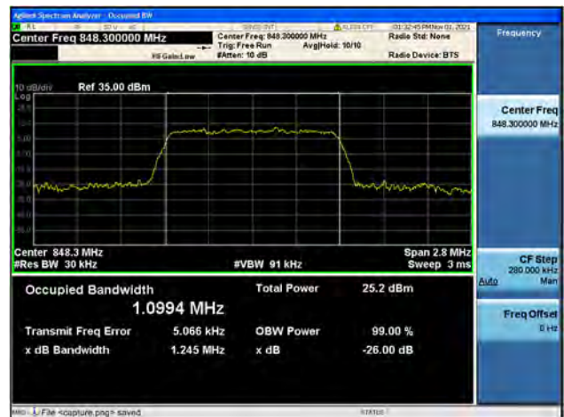
Band5 / 1.4MHz / High CH / 16QAM
