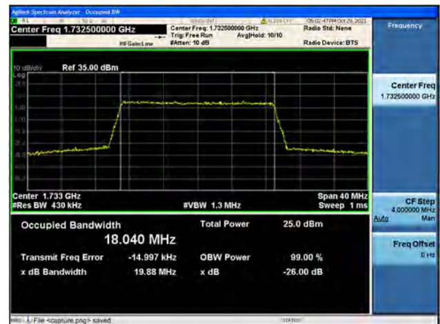
Band4 / 20MHz / High CH / 16QAM
