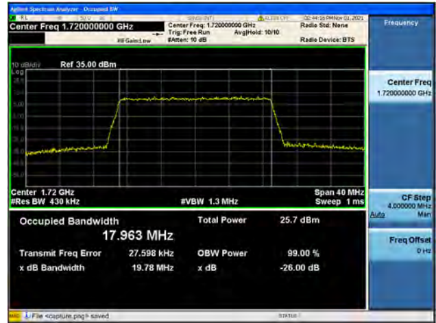
Band66 / 20MHz / Mid CH / 16QAM
