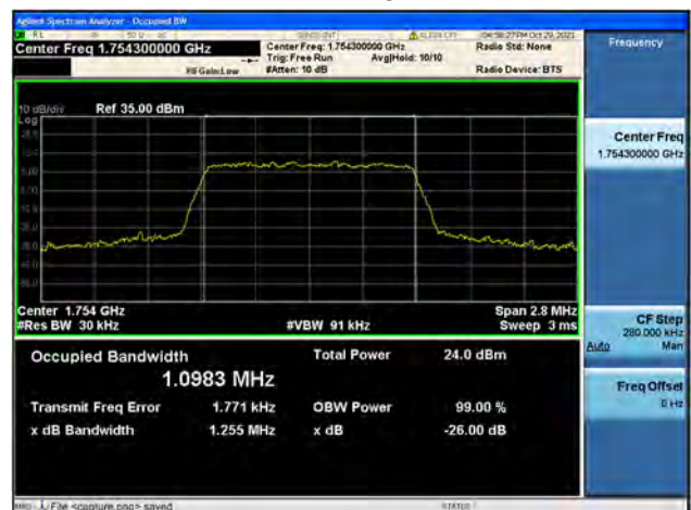
Band4 / 1.4MHz / High CH / 16QAM
