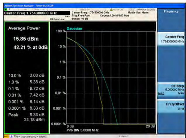
Band4 / 1.4MHz / High CH / 16QAM
