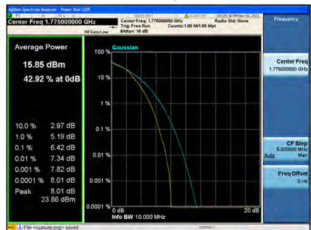
Band66 / 10MHz / High CH / 16QAM
