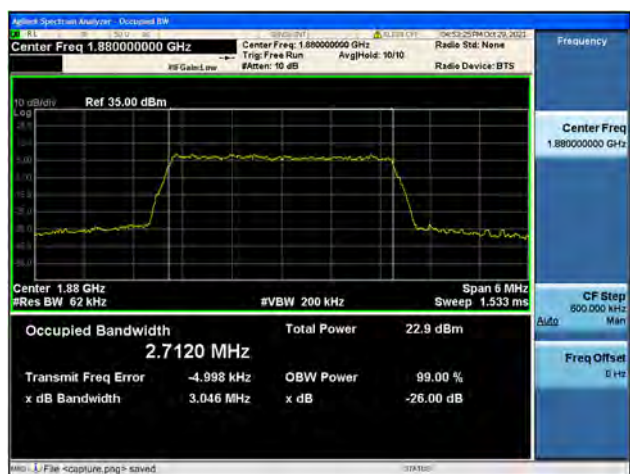
Band2 / 3MHz / High CH / 16QAM
