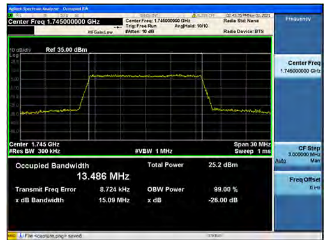
Band66 / 15MHz / High CH / 16QAM
