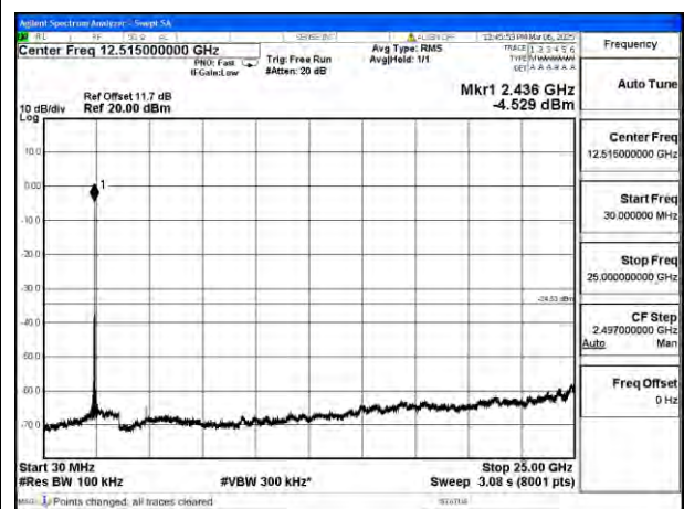
Mode:802.11n HT20 Frequency:2437MHz Ant:Chain0
