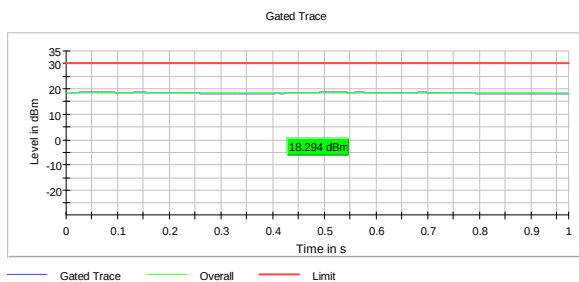
Output Power, 2437 MHz, 802.11b 1M
