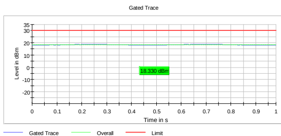
Output Power, 2452 MHz, 802.11b 1M
