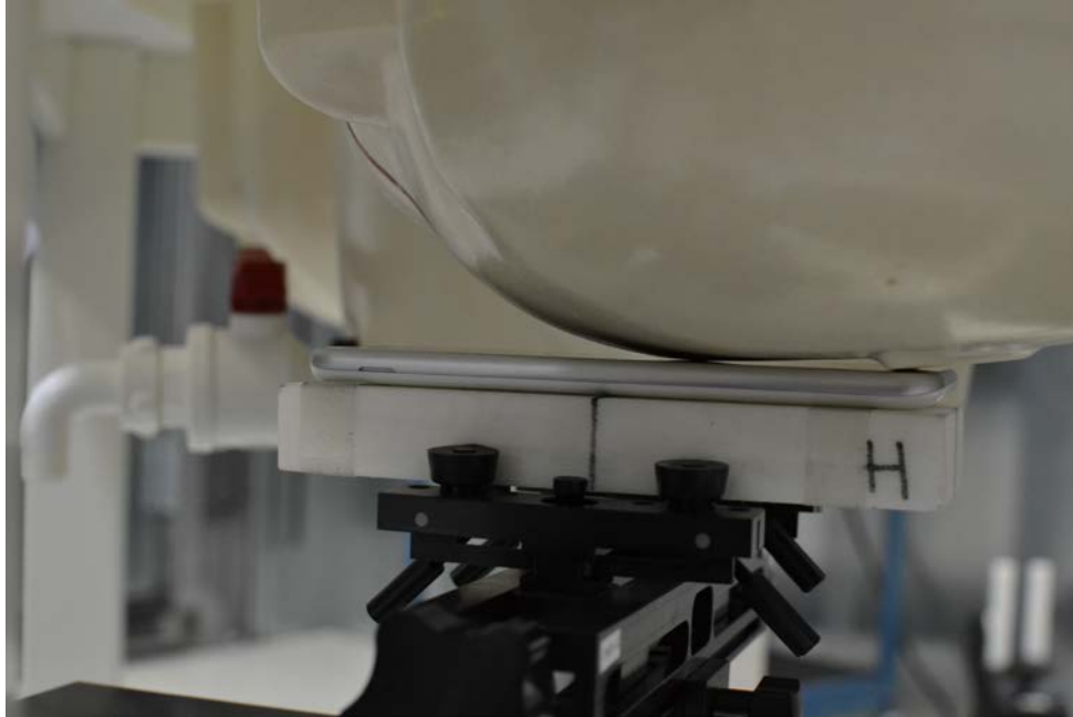
SAR Test Setup Photo 3: Left Cheek
