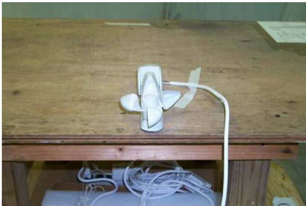
Figure 3.3 Radiated Test Setup, position 3-Z
