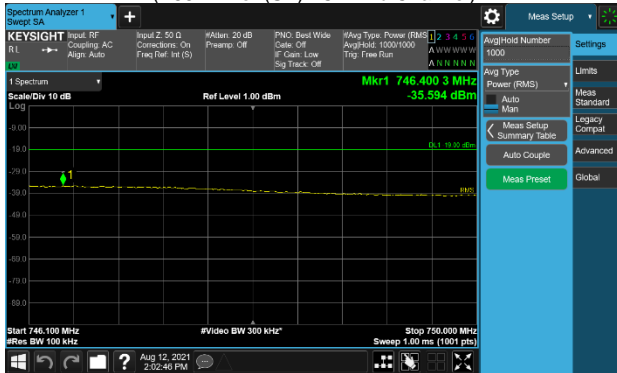
Plot 7-198. Conducted Spurious Emission Plot (746.1MHz to 750MHz) (B85 NB-IoT(SA) 1C – Mid Channel)
