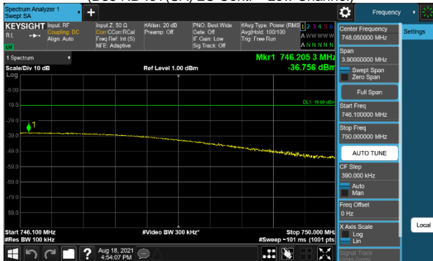
Plot 7-213. Conducted Spurious Emission Plot (746.1MHz to 750MHz) (B85 NB-IoT(SA) 2C Conti – Low Channel)
