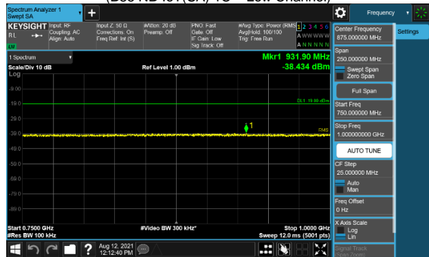
Plot 7-192. Conducted Spurious Emission Plot (750MHz to 1GHz) (B85 NB-IoT(SA) 1C – Low Channel)
