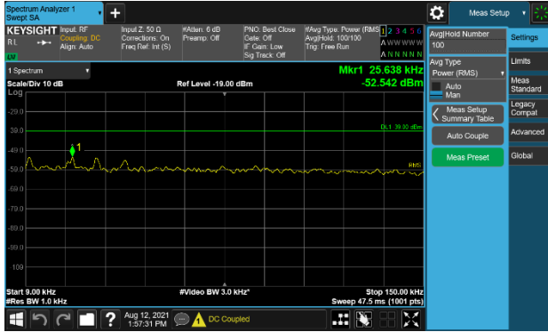
Plot 7-194. Conducted Spurious Emission Plot (9kHz to 150kHz) (B85 NB-IoT(SA) 1C – Mid Channel)
