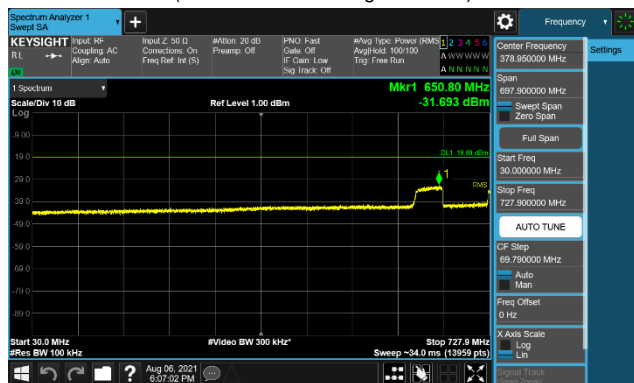
Plot 7-184. Conducted Spurious Emission Plot (30MHz to 727.9MHz) (B85 LTE 1C 5M – High Channel)
