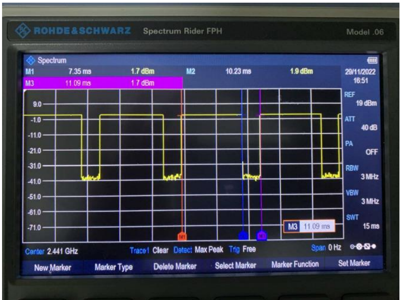
Time-domain plot for Bluetooth transmission signal
