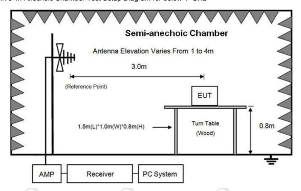
Semi-Anechoic 3m Chamber ANTENNA ELEVATION VARIES FROM 1 TO 4 METER 3m (Reference Point) 1.5m(L)\*1.0m(W)\*1.5m(H) EUT 1.5m TURN TABLE **ABSORBER** (FIBRE GLASS) AMP Spectrum Receiver PC System
