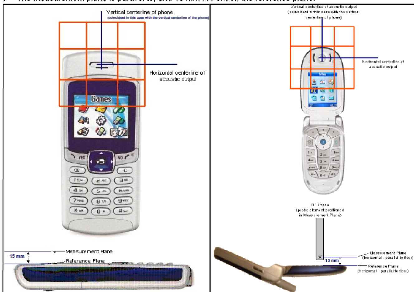
Fig.3 WD reference and plane for RF emission measurements
