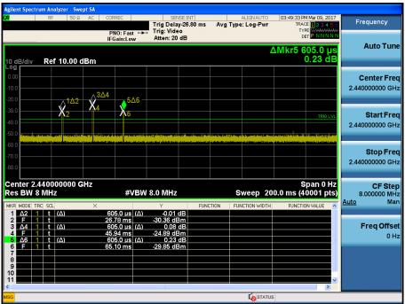
Note: Measure Duty Cycle = T / 100 ms ( T = sum of the individual on-time in 100 ms ) = (0.605ms + 0.605ms + 0.605ms) / 100 ms = 1.82%
