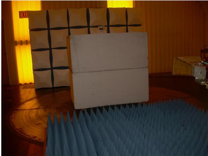
**Photograph 3: Front View Radiated Emissions Configuration – Above 1000 MHz**
