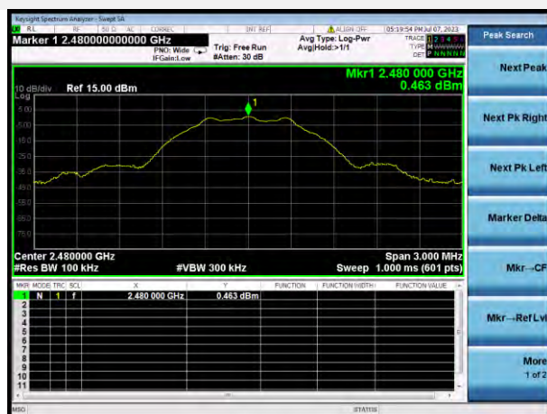
GFSK (BLE 1Mbps) HIGH CHANNEL, CARRIER LEVEL
