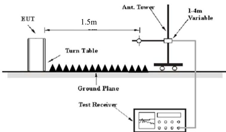
The radiated emission tests were performed in the 3 meters chamber test site, using the setup accordance with the ANSI C63.10-2013. The specification used was FCC 15.209, FCC 15.407, RSS-247, RSS-Gen limits.
