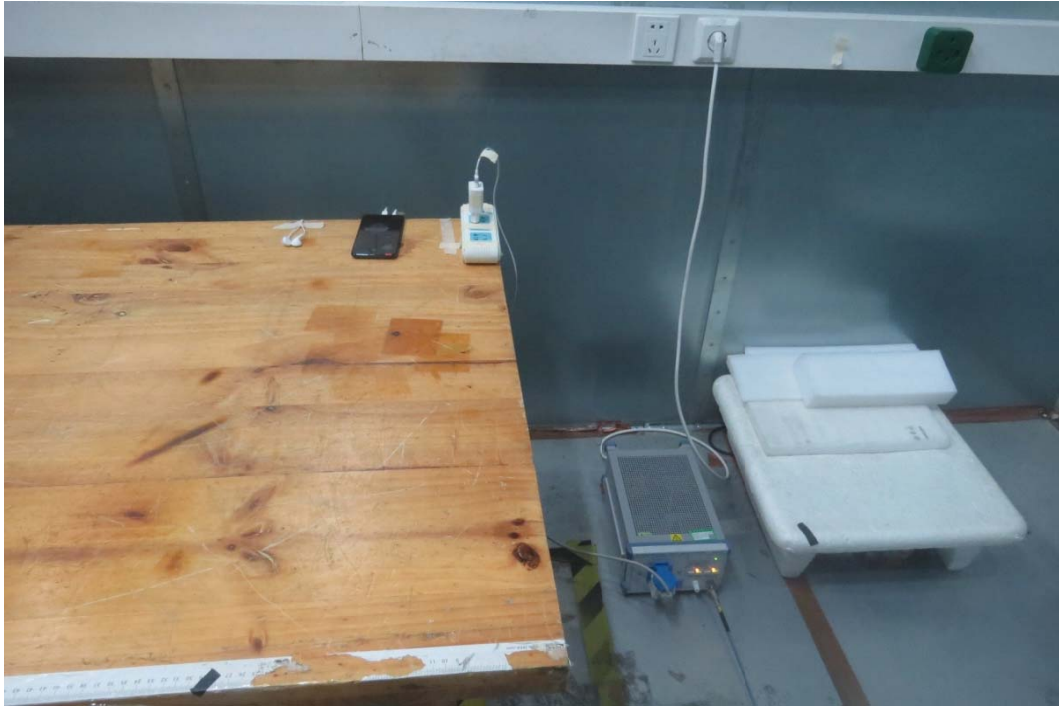
Picture 2 Conducted Emission Test Setup
