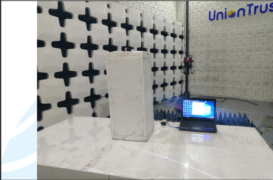
Radiated emission Test Setup (Above 1 GHz) -Left
