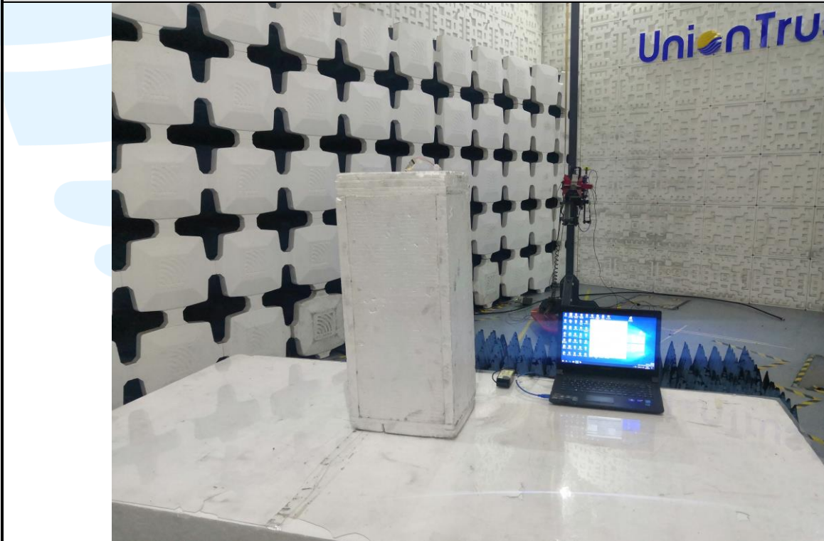
Radiated emission Test Setup (Above 1 GHz) -Right
