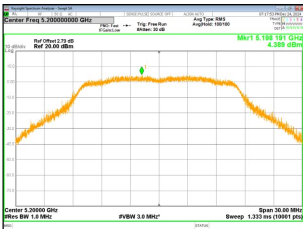
(802.11a) PSD plot on channel 40
