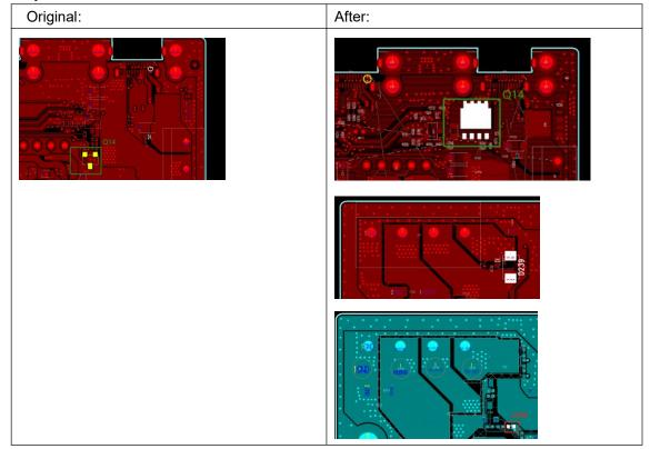
2. Auto transfer board: change IC from STM8S003 to GD32E230C8T6, add 24V to 5V/3.3V circuit, revise RS485 circuit, and adjustment on PCB
